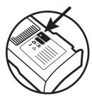
The battery pack's Active Status Indicator ("ASI") is located on the label face of the battery pack and is used to indicate battery pack status. A periodically blinking green LED indicates that the battery pack status is OK and the battery pack is ready for use. Absence of a blinking green LED indicates a battery pack problem or a depleted or missing 9V battery. Refer to the "Checking DDU-100 AED Status" section for information on battery pack LED indications.
